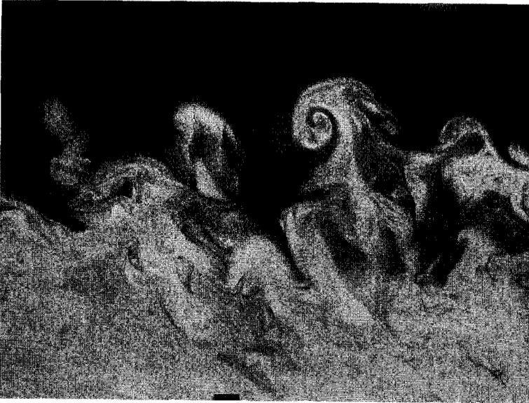
Fig. 1.2 Wind-tunnel visualization of large-scale structures in the outer layer of a turbulent boundary layer. Courtesy of M. Stanislas, IMFL, France.
