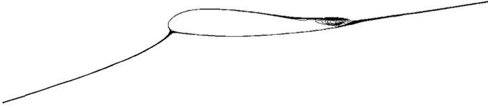
Fig. 3.11 Mean flow around the F2A wing: streamlines. The recirculation bubble on the suction side near the leading edge is correctly captured. Courtesy of H. Touil and J.P. Bertoglio, LMFA, France.
